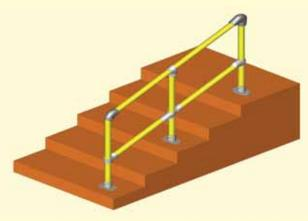
**KwikS3045** is a step section of 48.3mm diameter galvanised steel handrailing 3000mm long with three uprights and flat fix baseplates. The handrail accommodates variable step inclines from 30–45 degrees.
