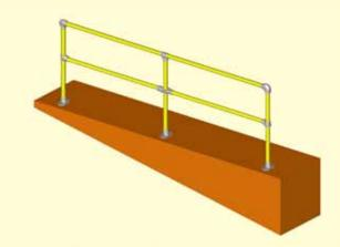
**KwikS011** is a ramp section of 48.3mm diameter galvanised steel handrailing 3000mm long with three uprights and angled flat fix baseplates. The handrail accommodates variable ramp inclines from 0–11 degrees.
