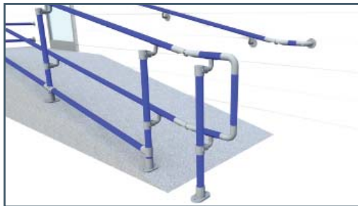
E) D RETURNS: Rail ends need to be rounded or return smoothly into a floor, wall or post.
