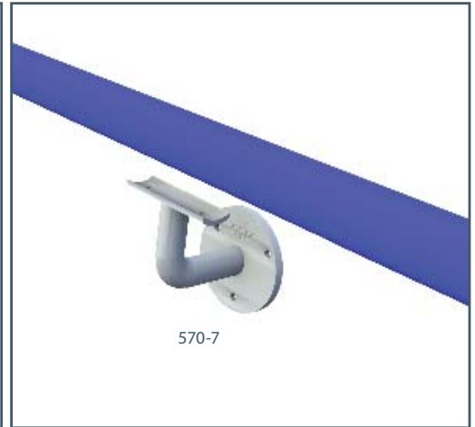
C) WALL MOUNT: The 570-7 is connected to the wall or wood posts using 6mm screws or bolts. The 570-7 is attached to the railing with No. 12 self-drilling screws or pop rivets.
