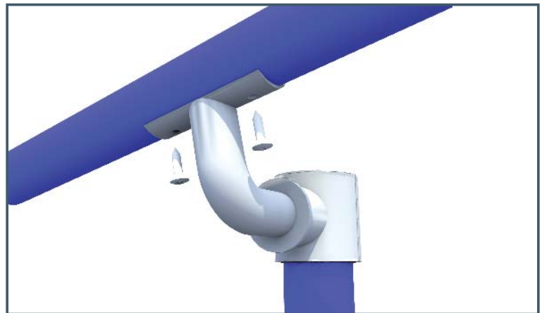
HANDRAIL BRACKET ATTACHMENT: Brackets attach to the handrail tube with two No. 12 self drilling screws or pop rivets. Use high quality hardware for the best results.
