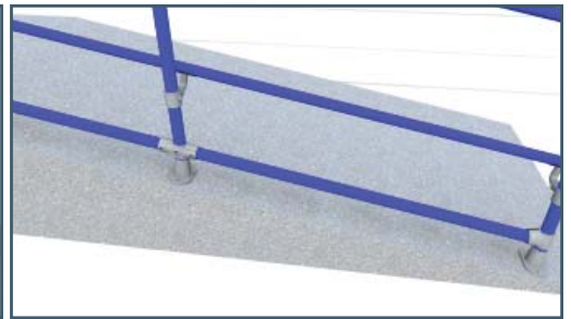
C) EDGE PROTECTION: When there is a drop off, ramps require a curb or curb rail to prevent wheel chairs from slipping out from under the railing. In some cases a mid rail is sufficient to provide this protection.
