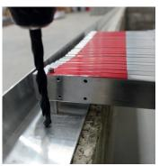
Remove spring loaded bolts if vertical location pin required. Allow enough depth for location pin to fully insert.
